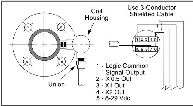
**Figure 5 – 1 Coil and 1 PA-6 Preamplifier**
