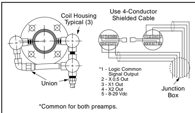
**Figure 7 – 2 Coils and 2 PA-6 Preamplifiers**
