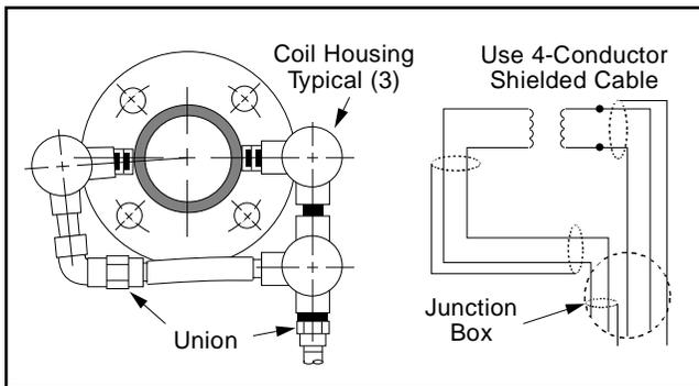
**Figure 6 – 2 Coils - No Preamplifier**
