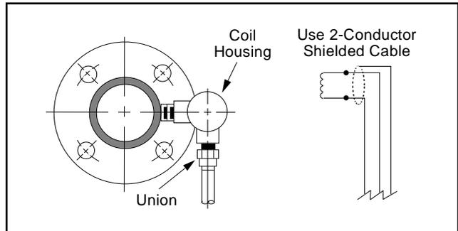
**Figure 4 – 1 Coil - No Preamplifier**
